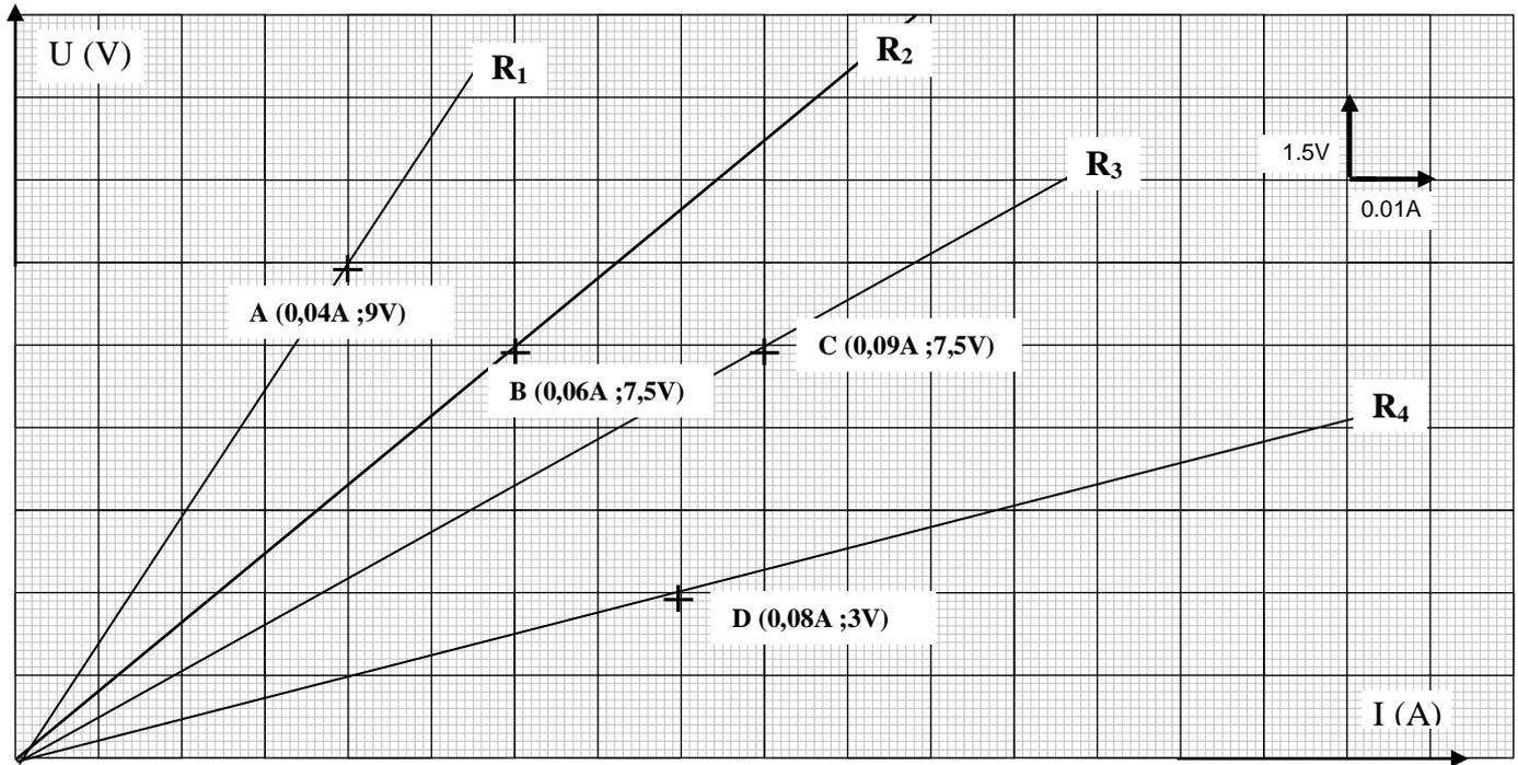
$R_1 = \frac{9}{0,04} = 225\Omega$  ;  $R_2 = \frac{7,5}{0,06} = 125\Omega$  ;  $R_3 = \frac{7,5}{0,09} = 83,34\Omega$  et  $R_4 = \frac{3}{0,08} = 37,5\Omega$
